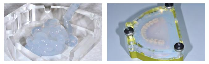
Figs 16 and 17 Transil F clear silicone was then injected through the openings on the upper flask half to completely fill the hollow of the assembled SR Nexco Flask.
